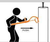
Push suspended objects utilizing the tool's concave head
