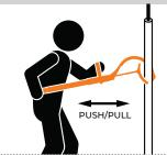
Capture and control suspended tubulars or cylindrical objects 3"-10" in diameter
